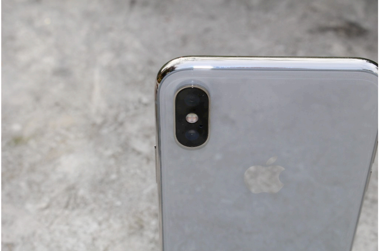
Dual cameras in vertical arrangement on iPhone X.
